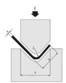
F[t] – pressure on 1m r – inner radius on steel b – minimum lenght of bending arm V – vee size
